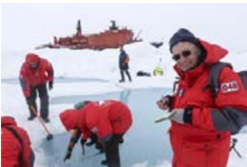
Figure 3. A group of passengers, led by a trained sea ice observer/expedition guide, measure depth and salinity of melt ponds at the Geographic North Pole, with icebreaker 50 let Pobedy in the background. These on-station measurements, combined with ship-based visual observations of ice coverage, thickness, floe size and topography during icebreaking contribute to the ASSIST6 (Arctic Shipborne Sea Ice Standardization Tool) Ice Watch data network and are also delivered to the Norwegian Ice Service to assist in ice charting.
